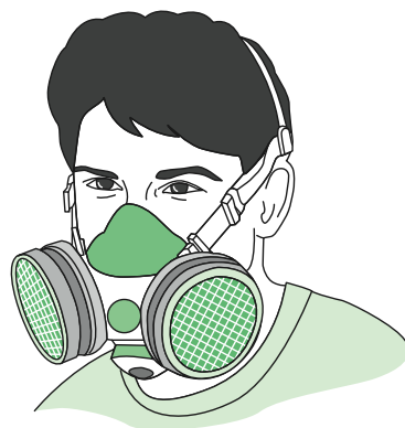
Half facemask chemical cartridge respirator (TC-23C).
