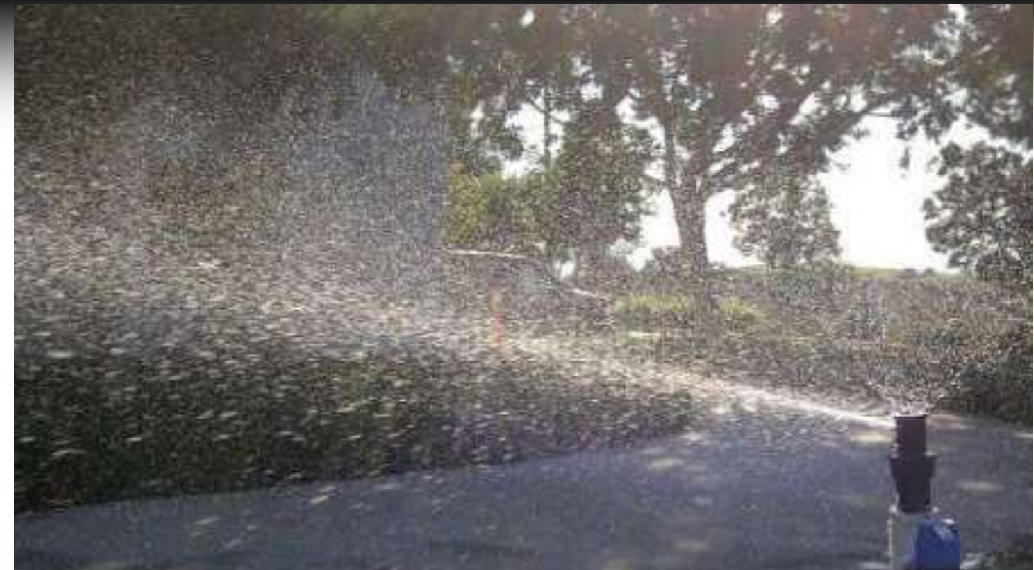
Toro Precision Spray with PCD 15H 1.16 GPM or 1"/hr. precipitation rate
