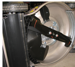
Figure 3. Rotary mower blade
