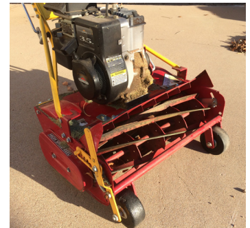
Figure 2. Reel mower blades
