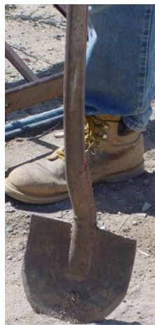
FIG. 33 MODIFIED SHOVEL FOR OFFSHOOT REMOVAL
